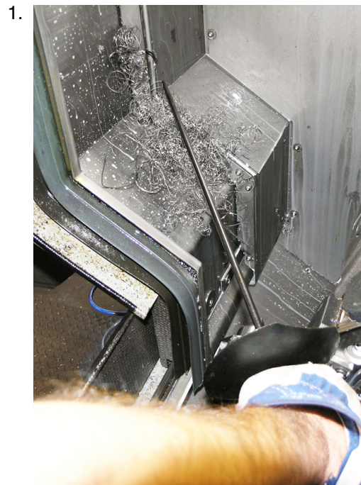
Example: 1 Removing chip nest using appropriate tools (e.g., chip hooks)
